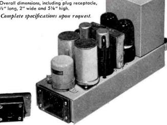
The Type 117-A has been designed as a program or monitor amplifier—gain 55 db. Operates from source impedance of 150/600 ohms and into load impedance of 150/600 ohms, in accordance with RMA proposed standards.
